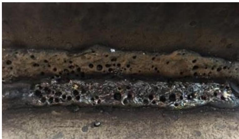
Fig. 3.2.27: Porosidade. Fonte: <https://www.mechanicwiz.com/porosity-in-welding/>
