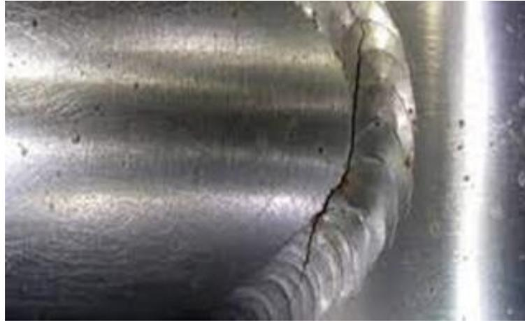
Fig. 3.2.28: Fissura. Fonte: <https://www.rapiddirect.com/blog/types-of-welding-defects/>
