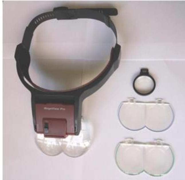
Figura 3.1.10. Lupas para exame macroscópico. Fonte: [https://sim.tuiasi.ro/wp-content/uploads/2021/05/Laborator\\_SM\\_2020.pdf](https://sim.tuiasi.ro/wp-content/uploads/2021/05/Laborator_SM_2020.pdf)
