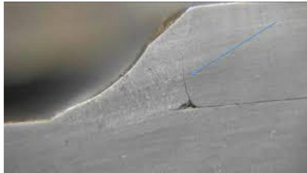
Fig. 3.2.29: Falta de fusão. Fonte: <https://www.onestopndt.com/ndt-articles/what-is-lack-of-fusion-in-welds>
