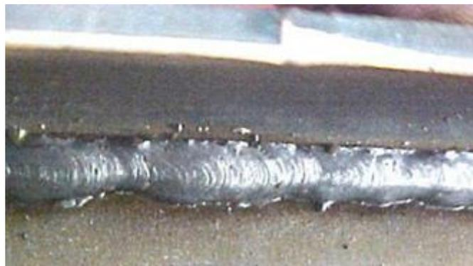
Fig. 3.2.30: Penetração incompleta. Fonte: <https://allgas.us/b/what-are-welding-defects--types-causes-and-remedies>
